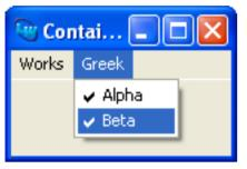
Note how the items in the menu component inherit the callback given to the parent, eliminating the need to specify a separate callback for each item or component in the menu.
