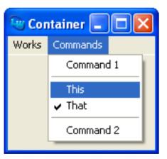
The menu items **This** and **That** are radio buttons, only one of which may be selected at a time. The other menu items are just ordinary commands, as you saw in the previous examples. Note that the CAPI automatically groups the items which are parts of a menu component so that they are separated from other items in the menu.
