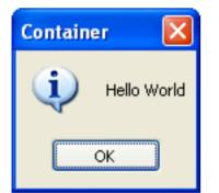
The CAPI provides the function <u>display-message</u> to allow you to pop up a dialog box containing a message and a Confirm button. This is one of many pre-defined facilities that the CAPI offers.
