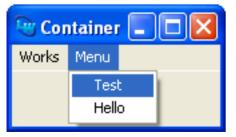
Remember that each instance of a menu item must not be used in more than one place at a time.
