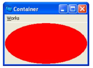
The <u>with-geometry</u> macro is used to set the size and position, or geometry, of the ellipse drawn by the draw-ellipse-pane function. The fill color depends on the radii of the ellipse - try resizing the window to see this. For more details of see the manual page for drawn-pinboard-object.
